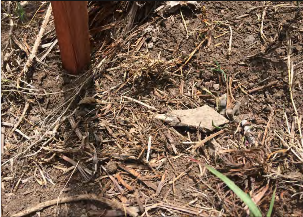
Photograph 13 – Identified bonded asbestos fragments within the fill of the dam in the eastern portion of the site, observed on the 12.11.2018
