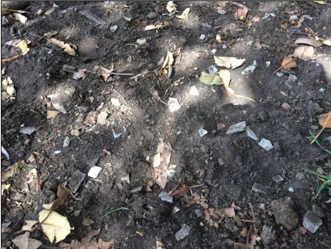
Photograph 11 – Bonded asbestos fragments identified in the eastern portion of the site, as observed on the 12.11.2018
