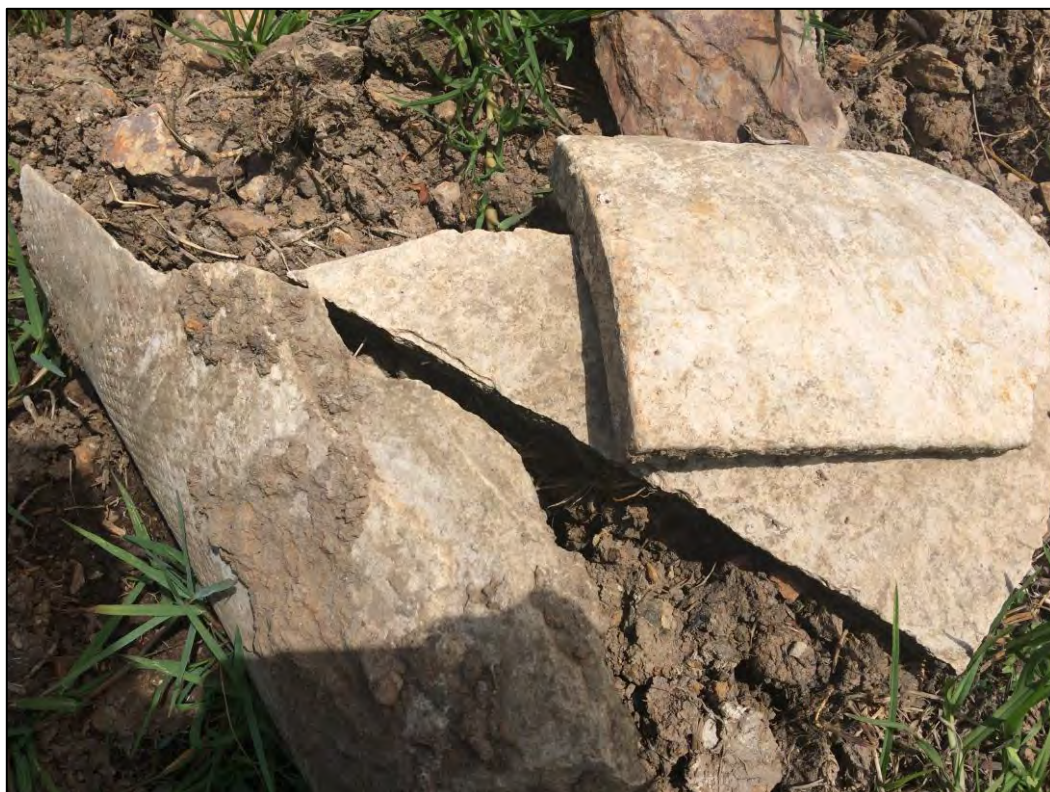
Photograph 10 – Bonded asbestos pipe identified in the eastern portion of the site, as observed on the 12.11.2018
